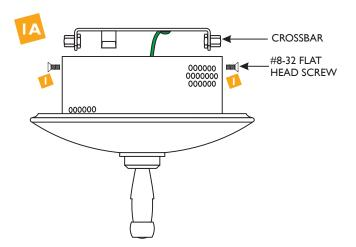
Remove the two #8-32 flat head screws to remove the crossbar.
